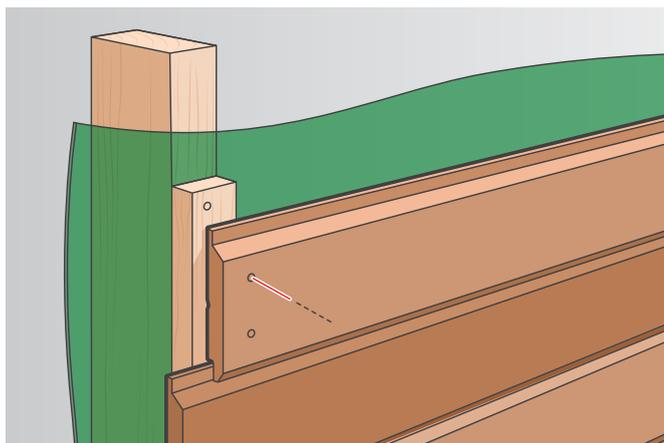
**Figure 1:** Preferred installation method for horizontal cladding showing:
