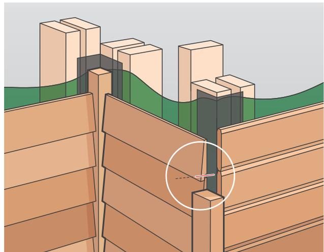
**Figure 4:** Traditional siding / weatherboards and VJ T and G cladding, using conventional corner stops. **This diagram shows:**
