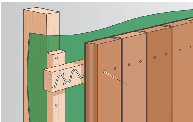
**Figure 2:** Preferred installation method for vertical cladding showing:
