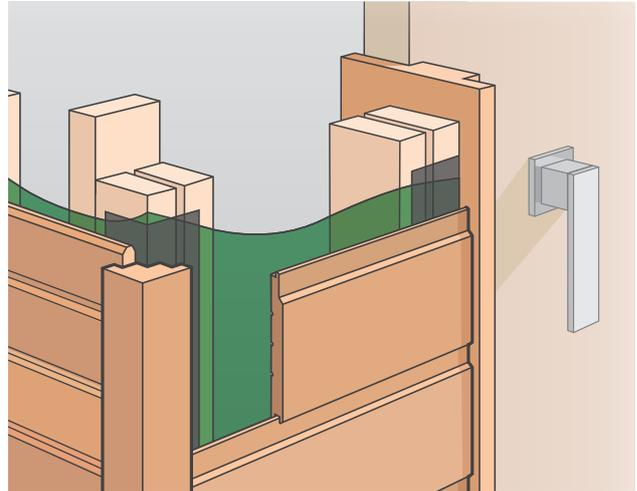
**Figure 3:** VJ and shiplap T and G cladding, using designer corner stops from Urbanline. **This diagram shows:**
