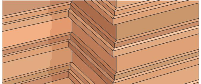
**Figure 5:** Mitred corners shown on Castelation® Stepped Combination. Urbanline recommends using external glue on all mitre cut corners to resist the corners opening up over time.
