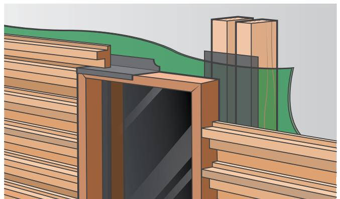
**Figure 7:** Flush finish window stop that frames the window. Window stop is DAR 91 x 30mm. **This diagram shows:**
